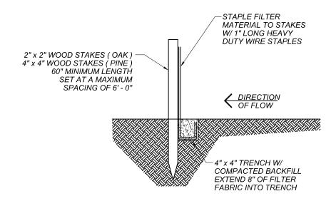
SILT FENCING SHALL BE EXTRA STRENGTH SYNTHETIC FILTER FARRIC HAVING A MINIMUM FLOW RATE OF 0.3 GAL/S.F./MIN. AND SHALL CONTAIN ULTRAVIOLET RAY INHIBITORS AND STABILIZERS OF EXPECTED USEABLE LIFE AT A TEMPERATURE RANGE OF 0 DEG. F. TO 120 DEG. F.
