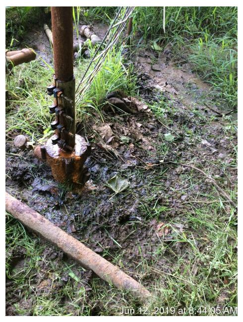
7-9-2019 Compliance Notice # 1536086906 follow up inspection. The injection tubing is leaking brine onto the ground. Contaminated area is approximately 8 feet by 4 feet. The well is fenced in with barb wire with no access to the well. The injection line is not connected to the injection tubing. Pillar has a service rig in the ERP field currently working on oil production wells.
