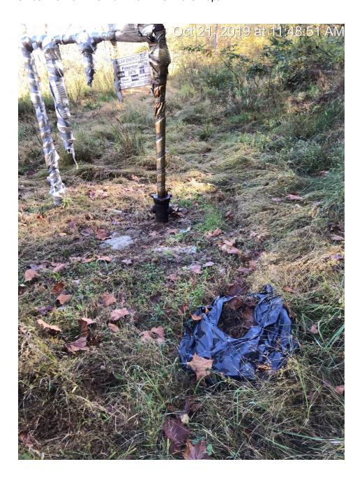
12-20-2019 Compliance Notice # 954126558 follow up inspection. Contaminated soil has not been removed from the location. Absorbent material has been applied to a 4 foot radius around the well. There is a black plastic trash bag with contaminated material, pads in it on site. The annulus is frozen.
